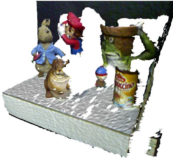
Figure 2.7: Example of a scene containing partial objects, caused by parts of their surface being invisible to the 3D scanner (scanned using a Kinect sensor by Tombari et al. [45]).
