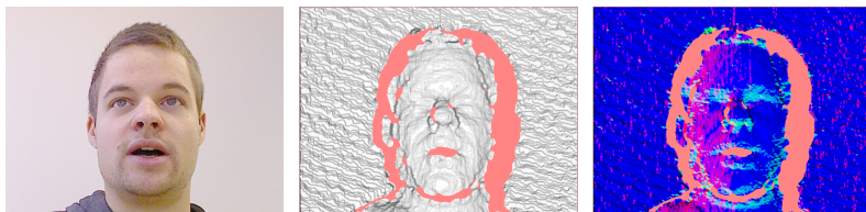
Figure 2.15: RGBD camera (Asus Xtion Pro) output: Left the RGB image, in the middle the Phong-shaded depth map and right the corresponding normal map (the red areas indicate that there is no observation).
