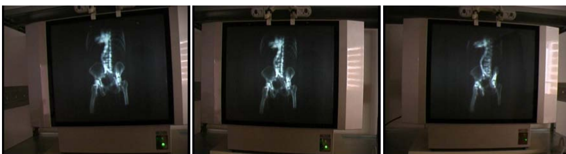
Figure 29: X-ray CT rendering. Direct capture from the spatial 3D display taken from different positions in order to immediately understand spatial information.
