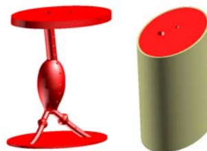
Figure 38: Aneurysm phantom realized at University of Innsbruck and used to validate the aortic measurement system.
