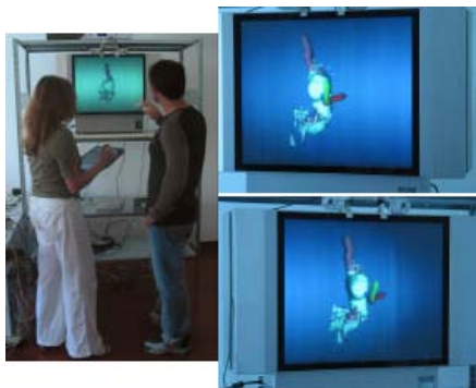
Figure 39: Left: the collaborative aneurysm analysis session: an operator selects and check measurement types, while the other interacts with the 3D model. Right: Aneurysm rendered on the holographic display, imaged at the same time from two different angles.
