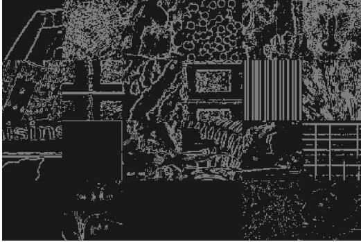
Fig. 3.3: Highlight of the \zeta effect by assigning a grayscale value 200 to pixels which have gradient count one, and a value 0 to other pixels.
