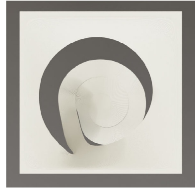
Figure 13: A sheet is pre-cut with an Archimedean spiral curve. Our MLS formulation enables exact cutting with complex crack geometry.
