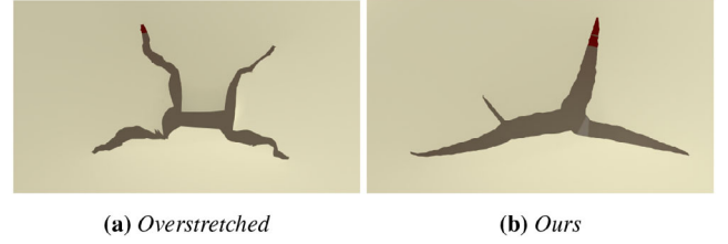
Figure 4: Extreme over-stretching (a) and our proposed method (b). Material near the crack is severely stretched when cutting a thin shell by the original phase-field method.
