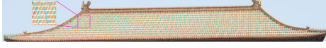
Figure 2: The tile direction field. The lines (colored in blue) indicate the tile directions at the sample points on the sample horizontal lines (colored in white).
