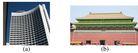
Figure 1: Interactive façade segmentation. (a) A hotel model. The user first draws the façade contour. (b) Meridian Gate. The user specifies necessary lines (colored in green) to segment the façade vertically, where the white lines are candidates with larger gradients.
