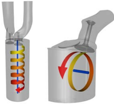
Figure 1: (left) The swirling motion of flow in the combustion chamber of a diesel engine. Swirl is used to describe circulation about the axis aligned with the valve cylinder. The intake ports at the top provide the tangential component of the flow necessary for swirl. The data set consists of 776,000 unstructured, adaptive resolution grid cells. (right) Some in-cylinder flows require a tumble motion flow pattern in order to mix fluid with oxygen. Tumble flow circulates around an axis perpendicular to the cylinder axis, orthogonal to the case of swirl motion.
