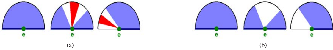
Figure 8: A 2D view of the shell of a grounded edge e ( e is perpendicular to the figure plane). (a) Disconnected tetrahedra from the ground are colored in red. They induce a singularity at e . (b) Configurations of a solid shell.
