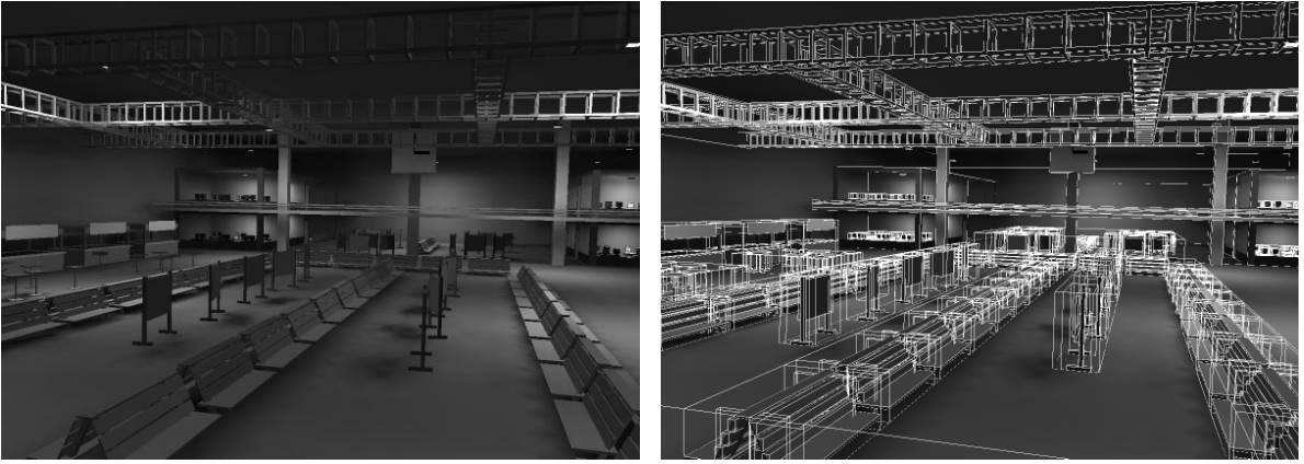
Figure 6: The model of a station consisting of approximately 32000 patches and 24 light sources. The lighting simulation based on clusters was computed in less than 10 minutes on a MIPS R8K CPU. Only 0.02 percent of the potential links were actually created (left). The image on the right shows the clustering hierarchy that was created.
