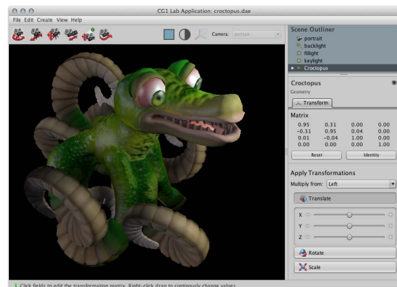
Figure 1: The editor of the course framework. This scene shows a model that has been exported from the game SPORE by Maxis using the COLLADA format. The matrix display is updated while using the widget in the transform panel.
