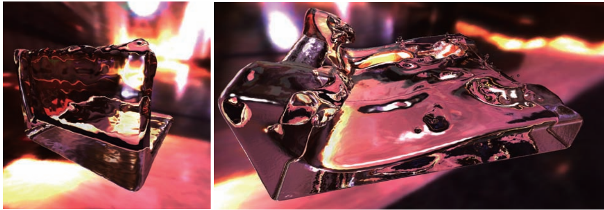
Figure 5: Left) Real-time rendering of 27,000 fluid particles with 64 * 64 * 64 grid; image size of figures is 512 * 512 . Even though fluid simulation is iterated 5 times with each frame, this program runs at about 30 fps, including density field construction, rendering, and simulation time. Calculating multiple refractions enables to see water through water. Right) Rendering of 1,000,000 particles with 192 * 192 * 192 grid. This is not real-time simulation (1.8sec/frame), but our method makes the density field construction 2.5 times faster. Background image from <www.debevec.org>.
