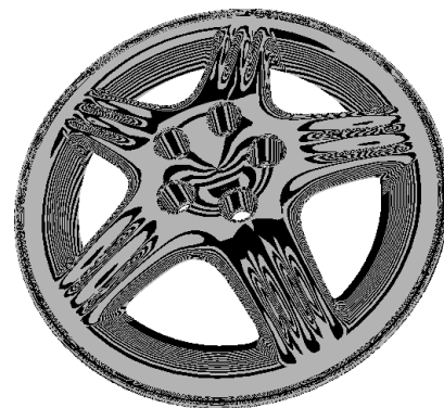
Figure 6: Wheel rim model rendered with isophotes (32 units).
