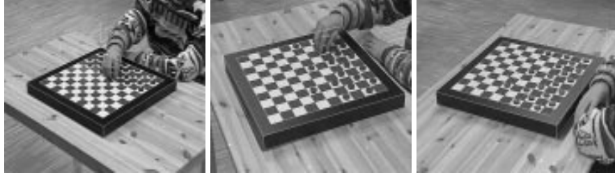
Fig. 4. Tracking results while rotating and translating the camera. The model's projection, drawn in white, remains perfectly superposed with the board. Note that the algorithm is relatively insensitive to occlusions.
