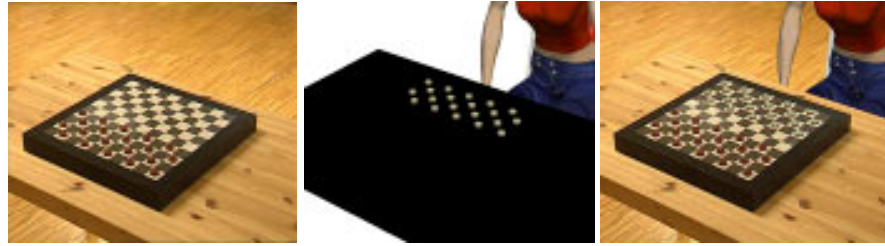
Fig. 7. Image compositing. Left: Real image with overlaid checker board model. Center: The synthetic image with black table for chroma-keying. In the actual system, the whole background is black but, in this image, we painted it white so that the table could be seen, Right: Composited image.
