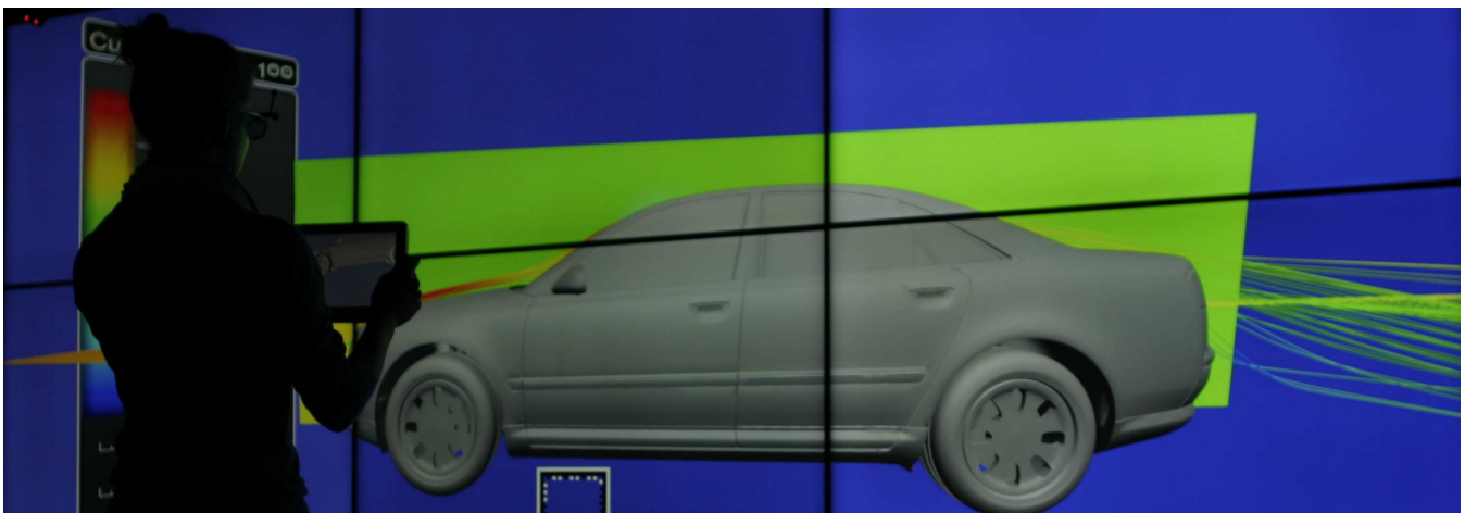
Figure 1: Interactive slicing of a CFD dataset using a tablet as spatial interaction device
