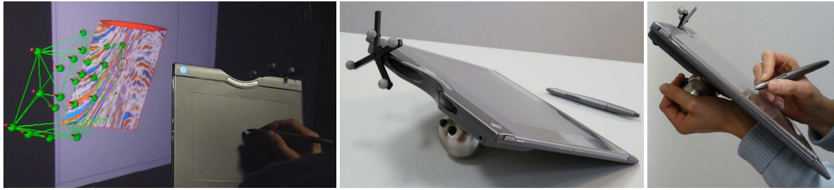
Figure 2: The 3D Sketch Slice is used as a prop for a volume slice to sketch uncertainties into volumetric seismic (left). It is equipped with spherical handle (middle), and comfortably rests on the user's forearm (right).
