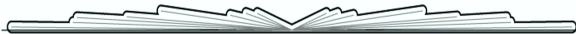
Figure 3: Side cut-away view of a single Nexrad radar. The 9 gray sweep lines are surrounded by regions of higher confidence in the accuracy of the readings. At lower elevations, spacing between the sweeps is close enough to assume readings from a continuous medium.
