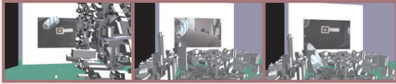
Figure 10: City plan model is detected by pattern 'B' and placed on the ground; SwissRe building model is detected by pattern 'A'; SwissRe building is placed on the desired empty area within the city plan
