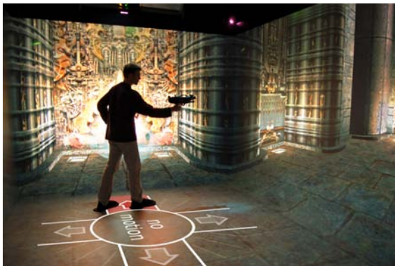
Figure 2: The user's head position controls the walk navigation speed in the game Quake III Arena . In this image the user moves sideways by standing left to the center. His hands are free for other interaction devices such as the gun. The bottom marks are overlaid for illustration purposes and are not visualized within the game.
