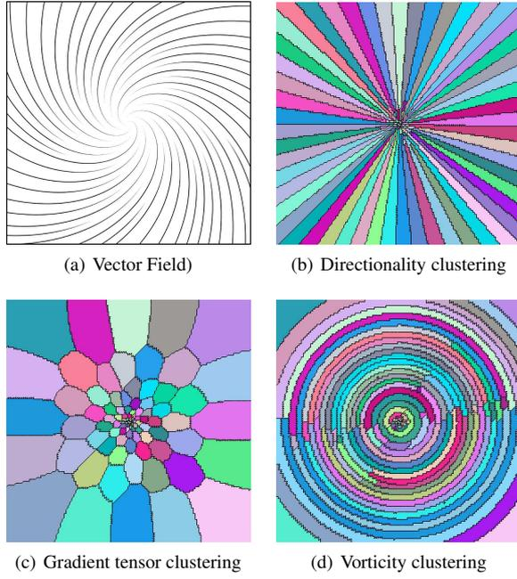
Figure 3: Application of various distortion metrics, 100 proxies.
