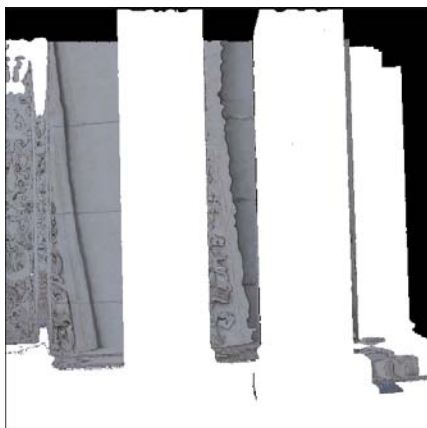
Figure 7: The results of mapping the scan when selecting correspondences from a dominantly planar region and using the camera projection computation. The extruded pillars are not mapped because the computed texture coordinates are out of bounds of the original photograph.
