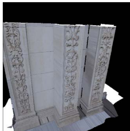
Figure 8: An angled view of the building scan mapped with the 2D homography. The mapping against the extruded pillars is done well. The sides the pillars are stretched since the original photograph in Figure 1c did not have the sides of the pillars in view.
