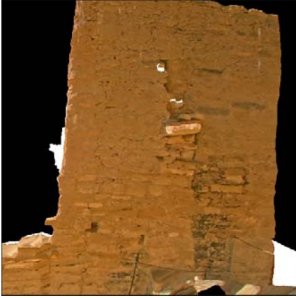
Figure 3: The result of texture mapping the adobe housing structure. Registration against the rocky, uneven surface of the building is done well. The floor region of the scan is not registered well against the photograph because of the lack of dominant correspondences to select from in the image.
