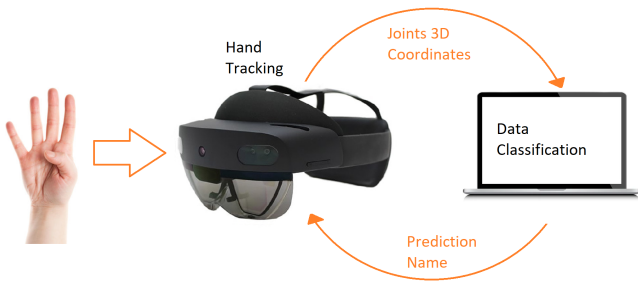
Figure 2: The client-server application: the HoloLens2 app sends the joints' stream to the PC and receives the classification results to be displayed.
