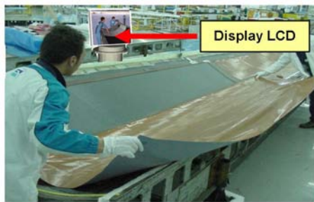
Figure 20: Development of the real operation with the aid of a digital handbook placed on a display near the tool.
