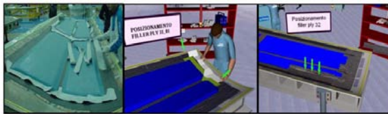
Figure 13: Filler ply stratification and immobilizing action on the honeycomb cores.
