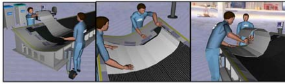
Figure 12: The ply kit components positioning and the protecting film removal.
