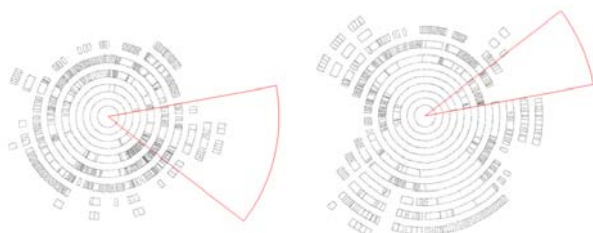
Figure 5: The angle may overlap two detail-resolution discs, hence two of these discs need to be cropped.
