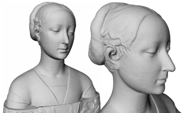
Figure 1: Sforza . Our variational method allows high-fidelity reconstruction of unprocessed point sets (3D scanned Sforza, 200K points). The final mesh is extracted via isocontouring of a scalar function computed through optimization.
