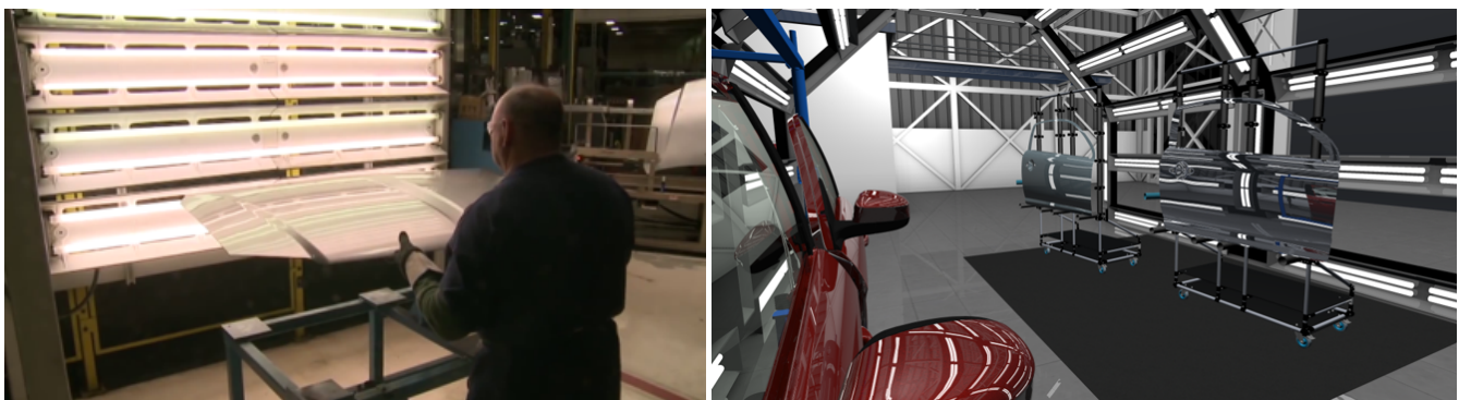
Figure 1: Left: Assessment of a physical prototype of a stamped metal sheet. Reflections of light tubes off a surface help detecting cosmetic shape defects that are difficult to quantify numerically. Right: Recreation of the light cage in a virtual reality setting, which eliminates the need for producing physical mockups.
