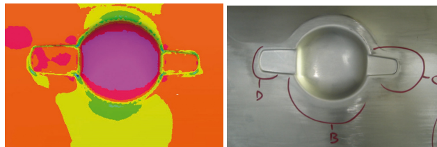
Figure 2: Methods for assessing surface defects. Left: Numerical simulation result as a contour plot showing normal distortion. Right: Result of stoning on a physical prototype panel, where scratch marks from a stone highlight localized changes in curvature. Structural defects are easily spotted, but it is difficult to say whether any distortion of the shape is aesthetically acceptable.
