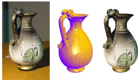
Figure 1: Left: a picture of the Greek vase model. Middle: a model reconstructed from several range images. Right: a synthetic view generated from the surface light field captured with our method. All acquired range images and pictures are registered in a fully automatic manner.
