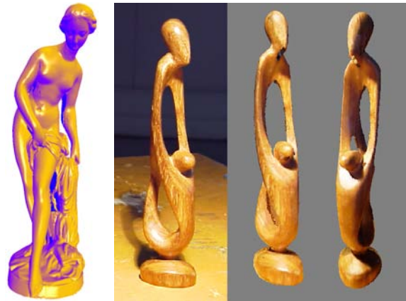
Figure 8: Left: the mesh of the Venus at Bath reconstructed from 23 range images registered with our method. Right: a picture of the African statue and two synthetic views generated from the surface light field acquired with our protocol.
