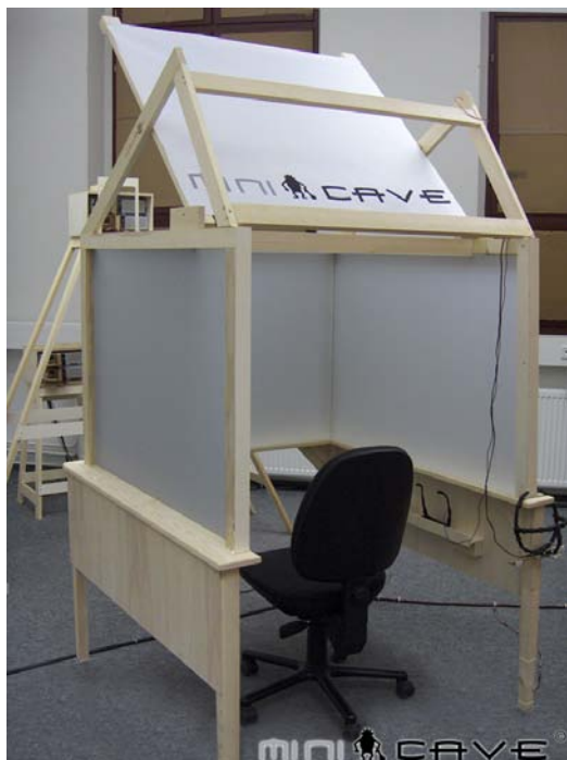
Figure 1: The CAVE frame in its final state. The tilted mirror guides the projection onto the top wall.
