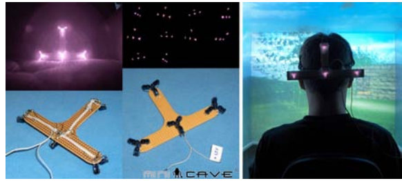
Figure 5: Headtracking setup for the miniCAVE. Four infrared LEDs are attached to a helmet worn by the user.
