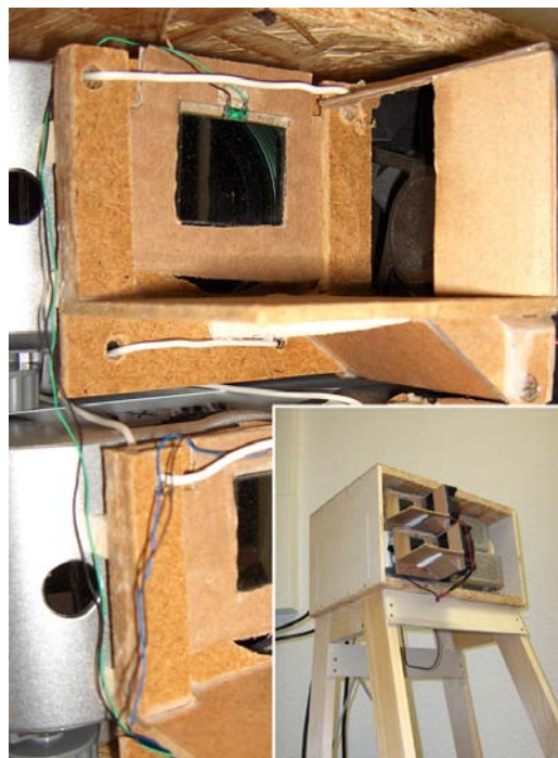
Figure 2: The projector stand (inset) and the mounting of the shutters used for stereo viewing.
