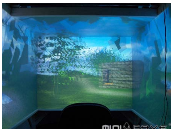
Figure 9: The CAVE viewer application presenting a scene in stereo mode on four walls.
