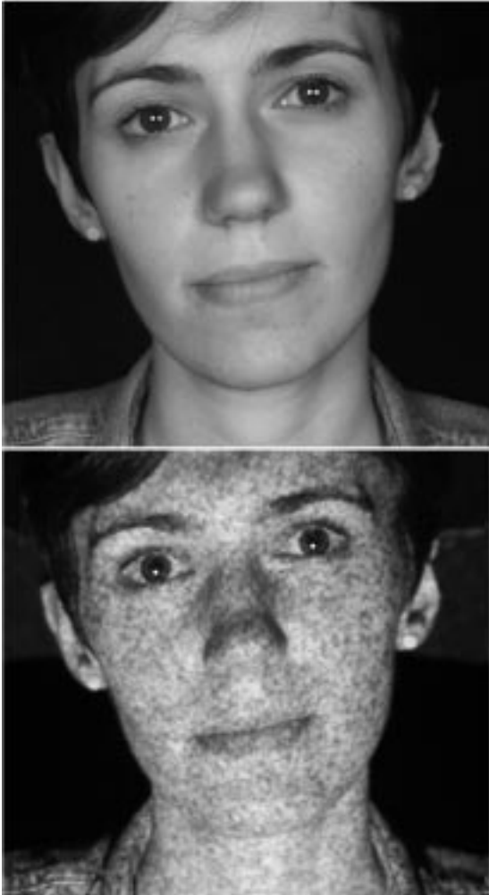
Figure 8: Example of 3D reconstruction of a face from three calibrated views. One of the original views used for texture mapping purposes (up); one of the views used for 3D reconstruction (down), obtained through projection of artificial texture (pseudo-random noise).
