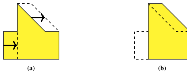
Figure 18: Area-preserving edge-move simplification [BMS11]. Contour polygon shapes (a) before and (b) after a single edge-move operation.
