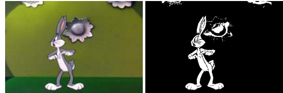
Figure 4: Segmentation with the SVM classifier model trained using 68 RGB samples from three images. This example shows the best classification of the Bugs Bunny character. Bugs Bunny is TM & ©Warner Bros. Entertainment Inc.
