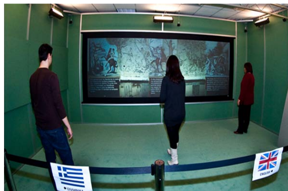
Figure 1: System overview. A display presents the artifact in its actual size and its content is updated based on the location and walkthrough trajectories of visitors, as estimated by a computer vision system. Based on these estimates the system presents graphical and textual annotations as well as a restored version of the artifact.
