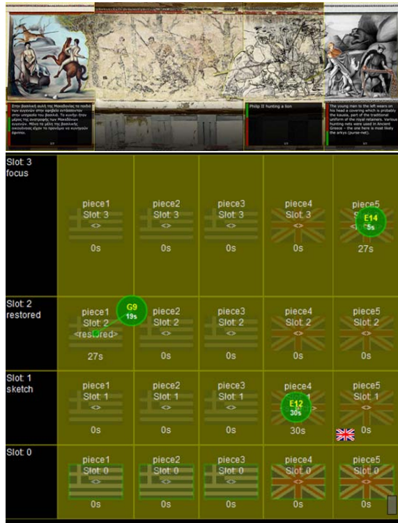
Figure 6: Modulation of projected content (top) based on user locations (bottom). The respective wall painting vertical slot changes, depending on the row and column that the user is located at. In the example the 2 nd and 3 rd slot from the left are inactive, as users are located at columns 1, 4 and 5. The matrix at the bottom corresponds to the spatial extent of the regions and the state of the application. Three users are in the room, represented by green circles. A flag on each column shows the active language on each slot of the display.
