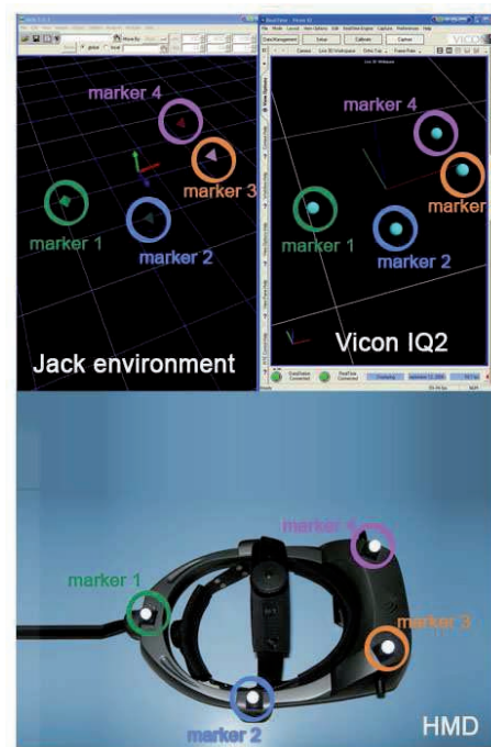
Figure 1: HMD marker positioning.
