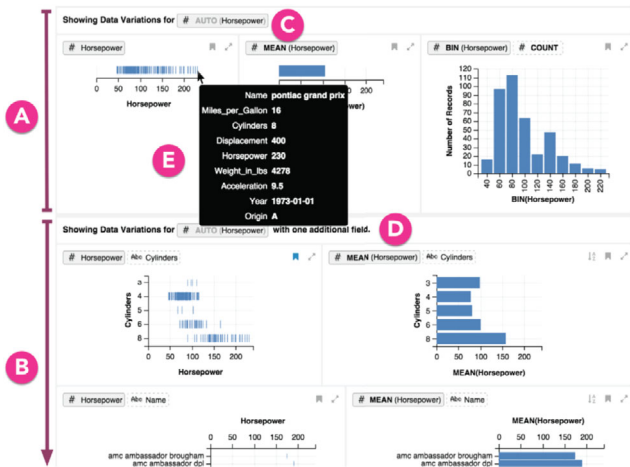
Figure 14: Example of directing guidance to the user by showing other visualizations of relevant data to the current state/query. By selecting a variable, the main gallery is updated showcasing: (A) the exact-match section containing multiple transformations and (B) the suggested section with the visualizations the system is recommending to the user [WMA*16].
