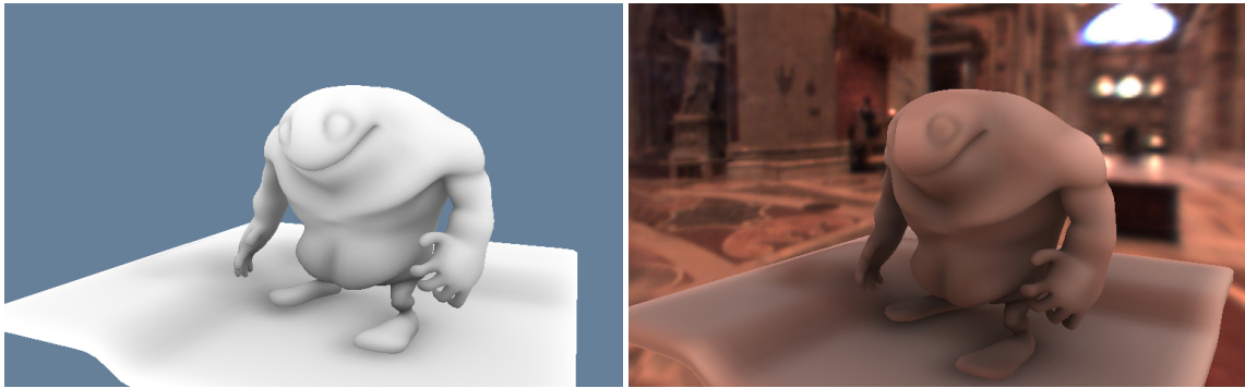
Figure 4: Comparison between ambient occlusion (left) and our anisotropic occlusion (right). Note that our algorithm generates more visually plausible shadow with comprehensive illumination environment.
