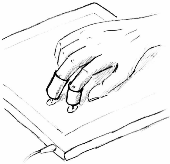
Figure 6: Specialized sensing devices such as thimbles equipped with small shoes may lead to an even more intuitive gait input via the graphics tablet.
