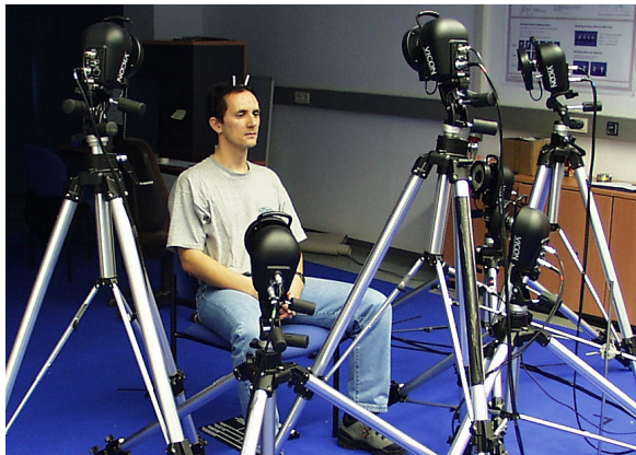
Figure 4: Camera setup for motion capture.
