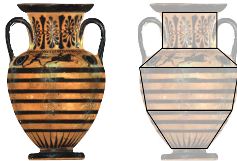
Figure 3: A vessel's shape can be approximated with several frustums which are rolled out separately (KHM Inv.-No. 3602).
