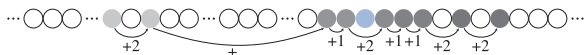
Figure 3: A typical set of neighbours computed on the sorted particles. The numbers indicate index differences in the sorted array. We propose a novel compression scheme to store the index differences.
