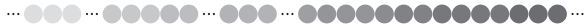
Figure 2: Particles sorted with respect to the cell index. Particles that share the same cell are adjacent in this list.
