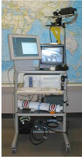
Left: The scanning rig used to acquire environments. Middle: A range scan registered with a color image. White lines are silhouette edges. Right: An item buffer resulting from warping a source image to the viewpoint of another source image with Z comparison. (McAllister, et al.)
