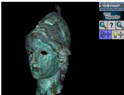
Figure 4: VIRTUAL INSPECTOR showing the Minerva head, rendered on the basis of the BRDF model sampled from the real statue.
