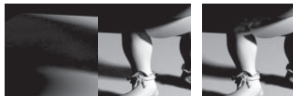
b) Light leaks when z threshold bias=0.05
