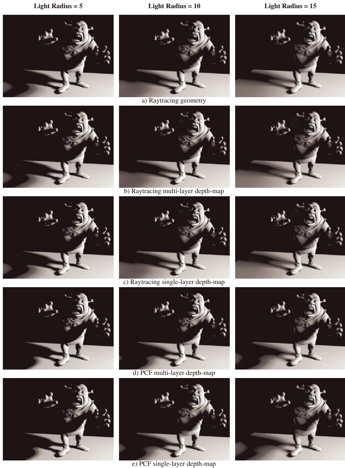
Figure 2: Shrek soft shadows: notice that the visual artifacts of soft shadows using PCF sampling and ray tracing of single layer shadow map grow with light size, while ray tracing MLSM generates shadows identical to stochastic ray tracing
