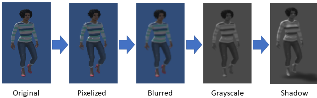
Figure 3: Shader processing of the 3D objects. The original image of the 3D model is first pixelized, then blurred in the horizontal and vertical direction using a Gaussian filter. The resultant image is then transformed to grayscale and finally, the shadow of the model is visualized on the transparent walking surface
