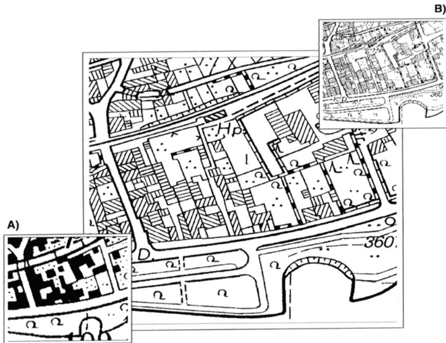
**Fig. 2-11:** Example of cartographic generalization [Hake02]: In the center a cutout of a 1:500 scale map. Part A shows the same cutout with a 1:25,000 scale. For comparison, part B is a reduction of the central cutout.
