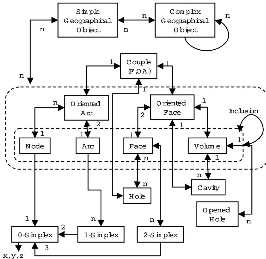
Fig. 3-8: de la Losa's 3D-GIS data model [LoCe99]
