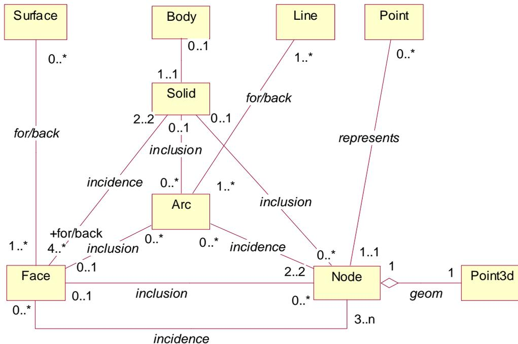
**Fig. 5-1:** Conceptual query-oriented data model in UDM
