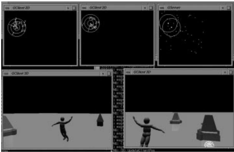
Picture 1: Demand-driven geometry transmission system view (server and two clients)
