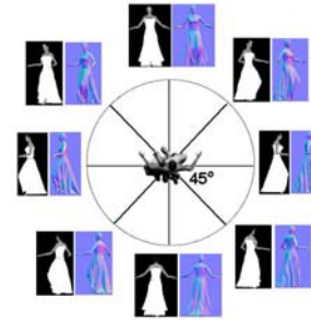
Figure 6: Generating impostor images from a camera positioned on the circumference of a circle every 45^\circ .
