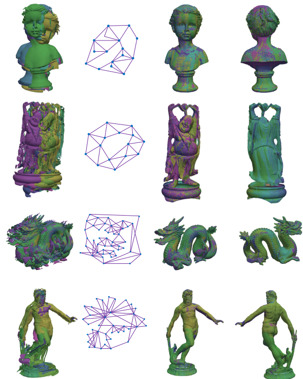
Figure 5: Registrations of real scanning range data. First column: initial states. Second column: graphs. Last two columns: the registration results from two viewpoints. Rows from top to bottom: Buste, Buddha, Dragon, and Neptune.
