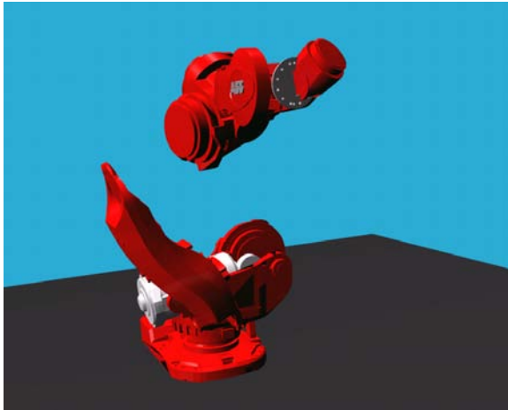
Figure 8: The kinematic chain breaks during the constrained movement.
