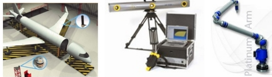
Figure 1: Tracking systems: (a) metris iGPS, (b) metris Krypton series, (c) FARO measurement arm
