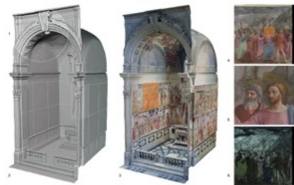
Figure 2: 3D model of the Brancacci Chapel: 1) wireframe detail; 2) segmented model; 3) textured model; 4) RGB texture mapping a segment; 5) texture detail; 6) Ultra Violet texture
