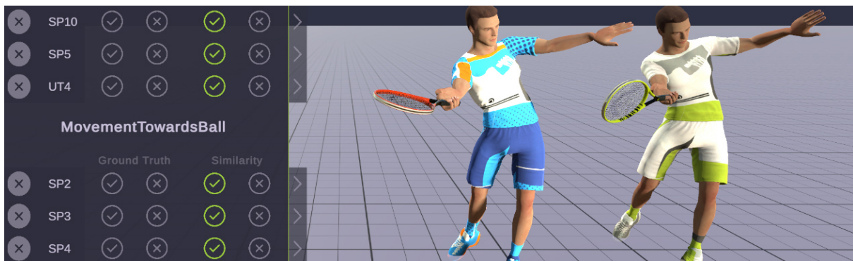
Figure 1: Visual feedback of the trainee's motion analysis by our method. The left panel shows correctness of performing individual training rules and the right window plays a 3D replay of the captured trainee's motion (blue) in comparison to a professional motion (green). These two motions are temporally aligned using dynamic time warping. When a user selects a specific training rule from the left window, a textual explanation of this rule is shown to help the user improve this specific aspect of the technique.
